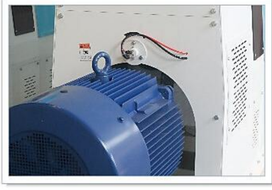
电机上下直拉, 调整简单 Motor adjustment is simple by straight pulling up and down
